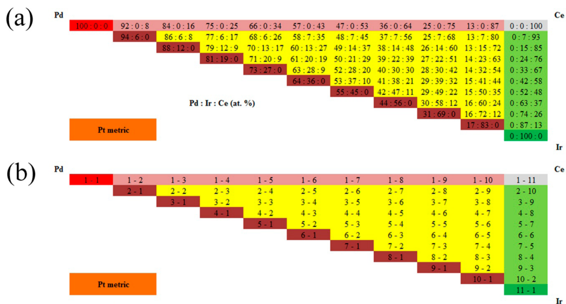
Figure 3. (a) Scheme of the compositions of combinatorial arrays for the Pd–Ir–Ce array. The ratios are expressed in Pd: Ir: Ce at. %. (b) Coordinates for each spot of the Pd–Ir–Ce array (x – y = line – order). Four Pt metric catalyst spots were included at the bottom left-hand corner as a reference to the performance of the prepared catalyst spots.
